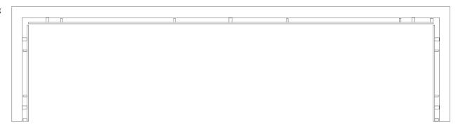
When measuring, first of all take the measurements directly into the corners of the bay for both the front and the side blinds. For the width of the blind for the front, reduce the corner to corner measurement by 90mm, this will allow for the 45mm space that is required either side. For the widths of the side blinds, reduce the corner to corner measurement by 45mm. Finally, order all three of your blinds as 'exact fitting'.
