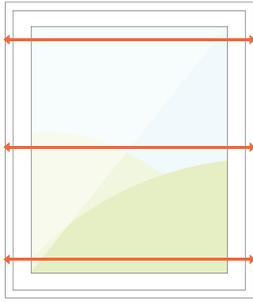
Take \*3 measurements from the outside edge of your window frame and choose the largest width. To your measurement, add 3.8cm for each side of the frame (left & right frame=7.6cm). This will be the width you use when placing your order on the website.
