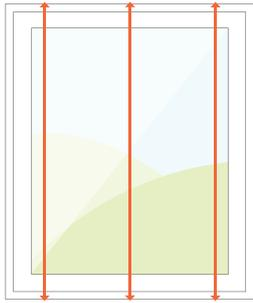
Take \*3 measurements from the outside edge of your window frame and choose the largest height. To your measurement, add 3.8cm for each frame (top & bottom frame=7.6cm). This will be the height you use when placing your order on the website.
