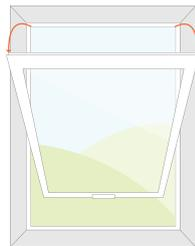
When determining the position which your shutters will sit within the recess, remember to take into account any obstructions such as handles or leverage on outward opening windows.
