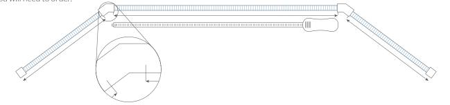
To establish your drop, measure from where the top of the blind will sit, down to where you want the blind to stop (normally the windowsill. Please deduct 10mm from the drop to ensure they do not drag on the windowsill.). With the measurements for the widths and the drops of your blinds, all you need to do now is enter them into our site and order them with an 'Exact' measurement type.
